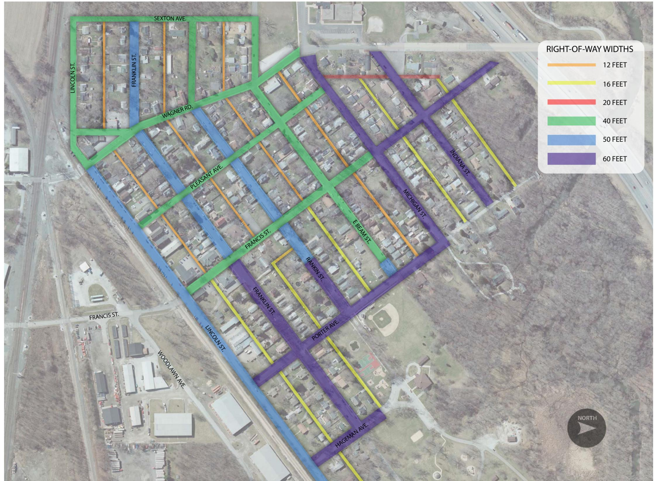
Figure 2-1. Right-of-Way Widths.
